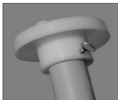
Figure 3: Attach the Cover Installer Tool onto the end of CPVC pipe.
